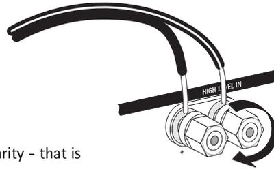
**NOTE:** When making high level connections be sure to maintain proper polarity - that is connect + to + (positive) to (positive) and - to - (negative) to (negative). All wire has one of its conductors marked in some way to make it easy to trace the connections. Typically there is a stripe on the insulation or a rib molded into it. Or the insulation will be transparent and the wire strands of one conductor will be copper colored and the other will be silver colored.
