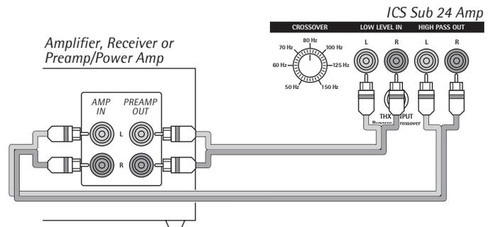
When using the low level connections, the signal from the High Pass Outputs that is returned to your amplifier is high pass filtered to remove sound below 80Hz. This is a non-adjustable filter. It is not affected by the setting of the Crossover control. See the Fine Tuning section of this manual for more information.
