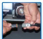
Used with the Siemens "Smart System", proximity switches are used to monitor various machine functions.
