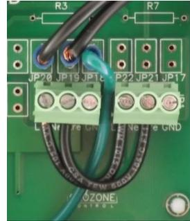
3. Pass the 120V trigger wire through the smallest strain relief and connect the conductors as follows:
