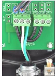
**\*Make sure to keep the jumpers between JP1 and JP4 hooked up as shipped from factory**
