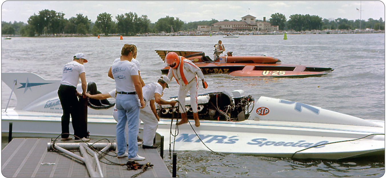
By 1969, much weight and the arrow-feather tail were removed and the boat was given a more conventional look and a new name. In the background is the catamaran Pride of Pay 'N Pak , which used a design that also was trying to discover more stability.
