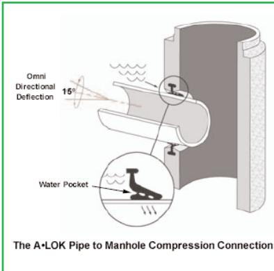
A-LOK X-CEL connectors prevent infiltration and ex-filtration into wastewater or stormwater systems, and are installed in the precast structure in a way that does not require coring or placement after the base component is cast. This eliminates residual waste from coring, disposal of the slugs or wasted raw material utilization or energy. Once cast-in, the connector becomes an integral component of the structure wall.
