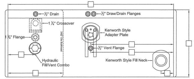
Please note: All sizes are NPTF unless otherwise noted and reference all measurements from the lateral weld seam and the end cap weld seam to the center of the fittings. South Towns Specialties, LLC
