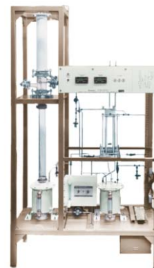
Model H-6160 Solid-Liquid Extraction Demonstrator Dimensions: 80"H x 45"W x 20"D
