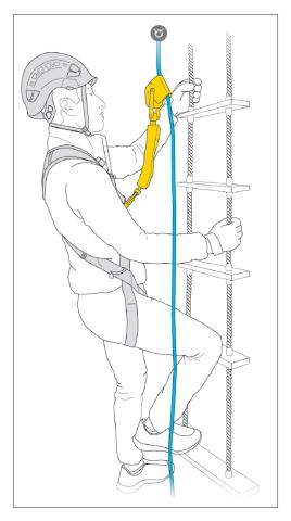
Petzl's **Maritime Pilot Ladder Fall Protection Kit** is a temporary vertical lifeline system certified under the ANSI Z359.15 standard and designed to protect a user during ladder climbing and descending should a fall occur.
