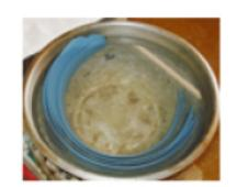
Step 5: Insert the fastener. From here on, gloves are recommended to be worn as the straps can be very hot coming out of the water. Remove one strap with a pair of tongs. Insert rivets into both ends of the strap.
