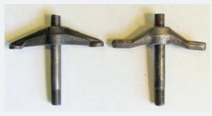
By reversing the later design clamp, it can be used on a block with the earlier, longer studs.
