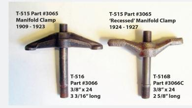
The manifold clamp underwent a design modification in 1924 to a 'recessed' design with double surface pads for the exhaust and intake manifolds. This part kept the same part number and factory number, likely due to its universal application. The recessed type can be used with either the short studs or the earlier longer studs by just installing the clamp inverted.
