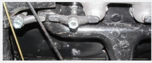
Later recessed clamps reversed and fitted to long studs.
