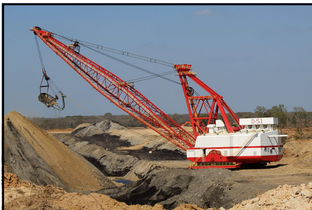
A dragline excavating phosphate.
