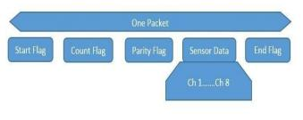
Fig. 6. Wi-Fi Frame Algorithm
