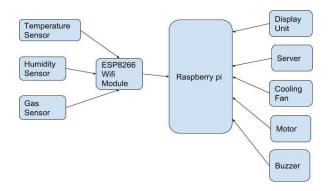
Fig. 1. Block diagram of WSN system
