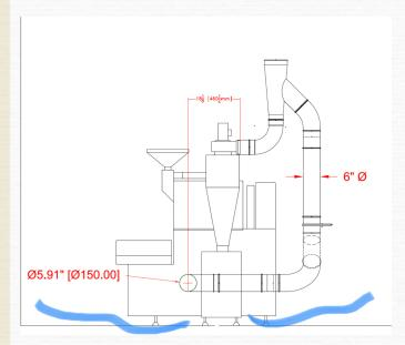
AS SEEN IN ILLUSTRATION OF FRONT VIEW ON THE BC-1 THRU 5 AIRFLOW INTO ROASTER IN PART COMES THROUGH THE BOTTOM OF UNIT AND MUST NOT BE COVERED OR BLOCKED IN ANY WAY.
