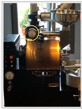
USING A MAG AIRFLOW GAUGE (SUCH AS THE ONE IN IMAGE ABOVE) WILL HELP YOU TO KEEP TRACK OF PROPER POSITIVE AIRFLOW THROUGH ROASTER AND EXHAUST
