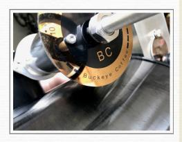
DAMPER HAS OPENINGS RANGING FROM 1-10. MOST ROASTING BEGINS WITH LOWER AIRFLOW (2-4 DURING DRYING PHASE) THEN INCREASES DURING BROWNING OR MAILLARD PHASE (4-6) AND MAY INCREASE MUCH HIGHER DURING ROASTING PHASE(6-9) DEPENDING ON
