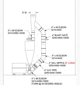
**ABOVE ILLUSTRATION IS JUST FOR GENERAL SETUP. PIPE SETUP AND** SIZES VARY DEPENDING ON **ROASTER**
