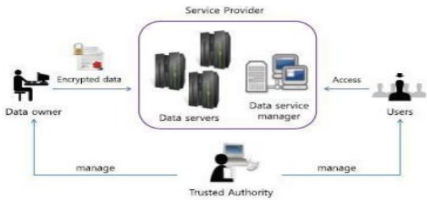
Fig .4 :Architecture of Data sharing System
