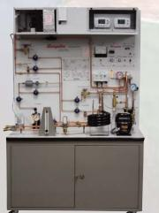
The Hampden Model H-RST-12 Heat Pump Trainer with water cooled condenser provides the student with an introduction to the principle components of heat pump systems.
