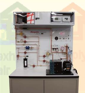
The Hampden Model H-RST-8 Heat Pump Trainer provides students with an introduction to the principal components of heat pump systems.
