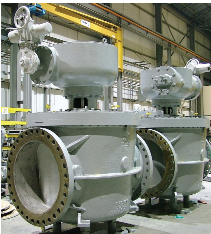
City of Detroit Water, Michigan, USA — Remanufactured 36" Allis Chalmers Rotovalve with electric motor actuator
