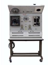
The **Model H-EH-2A** includes the following: Radiant Ceiling Lamp, Radiant Ceiling Heater, Radiant Ceiling Panel, Forced Air Wall Heater, Radiant Baseboard Heater, Low Voltage Transformer Relay, Low Voltage Thermostat and Line Voltage Thermostat.
