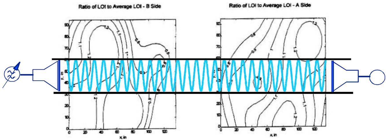
**Duct Gas / LOI Stratification Is Not a Problem When Instrument Is Not Dependent On Point Sampling**
