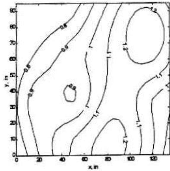
Typical Gas Distribution In Exit Gas Outlet Duct : 40% Variation Across Width of Unit
