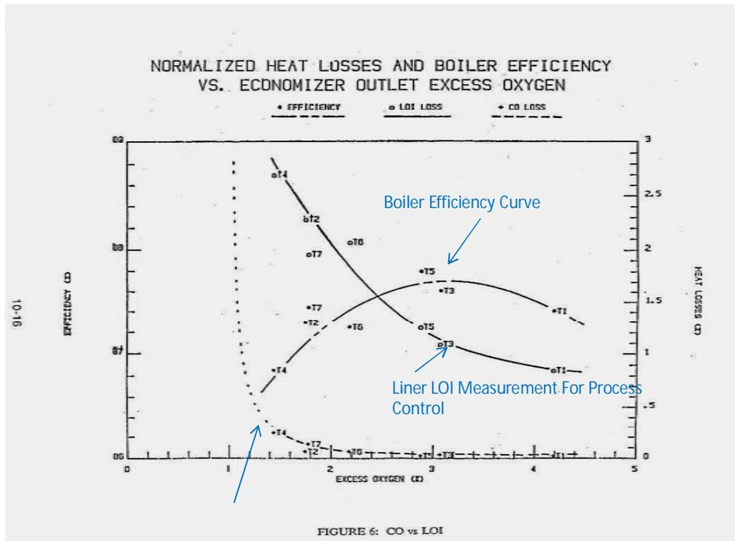
Non-linear & low sensitivity CO measurement, unsuitable for process control
