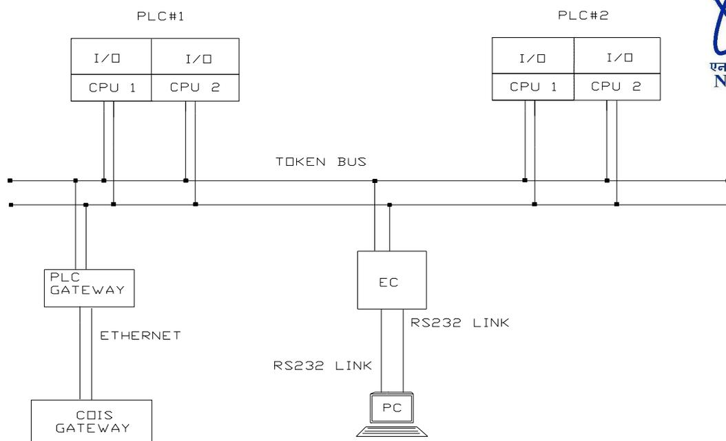
PLC ARCHITECTURE WITH REDUNDANT I/O AND REDUNDANT PLCs
