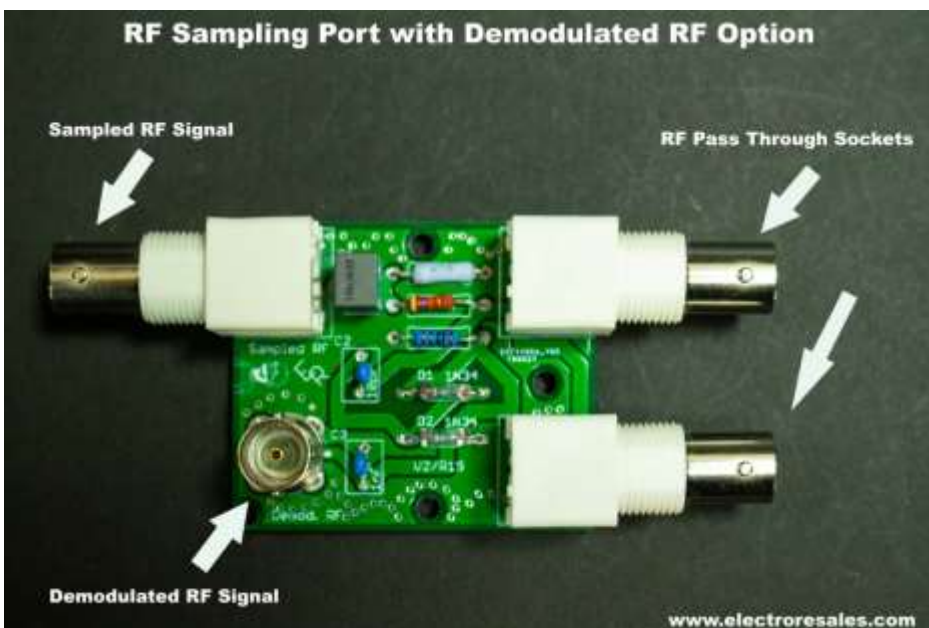
Image 1 - The Sampler with key parts noted
