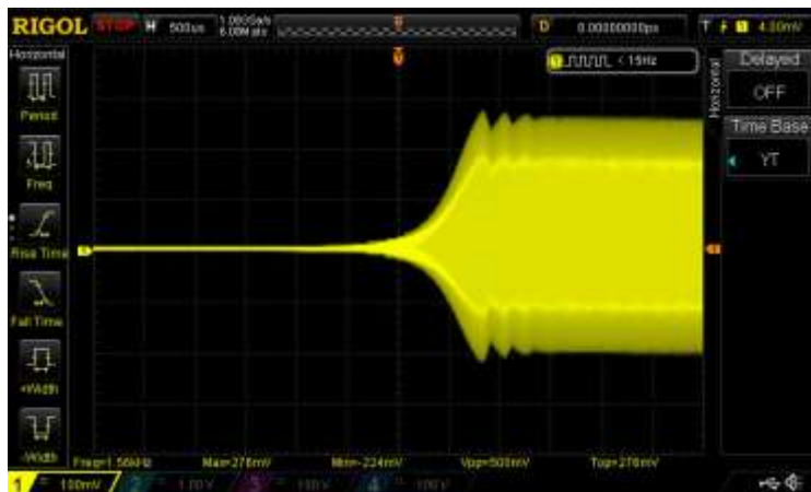
Image 3c - Two Tone signal with SSB input
