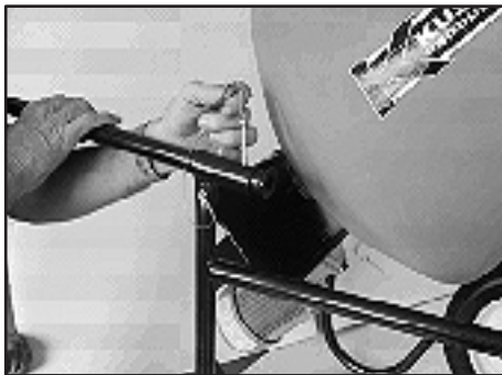
Step 7 - Slide handles in place, secure with lock pins / lanyards and install grips
