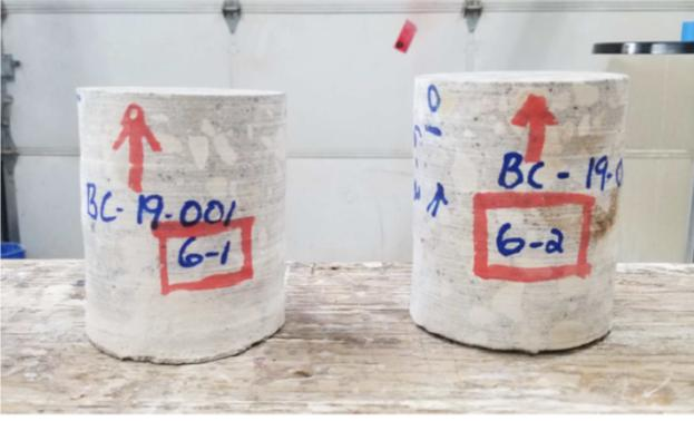
*Figure 1 - Roofing concrete cores without MVRA, samples 6-1 and 6-2*
