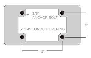
Standard Concrete Foundation or Optional Screw-In Bollard Foundation<sup>(1)</sup>
