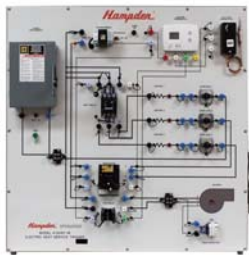
The Model H-EHST-1B Electric Heat Service Trainer facilitates the study and troubleshooting of the electrical and control circuits of an electric heat furnace.
