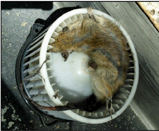
Rat that got trapped inside blower motor under hood. Owner noticed a bad odor and this is what we found.
