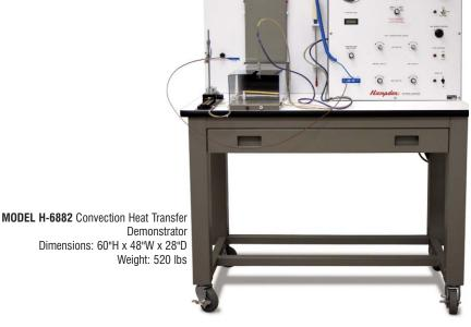
accuracy of  $\pm 2\%$ . There are also four power rheostats for fine adjustment of the temperature profile of the test device. Finally, there is a fan motor speed control which determines the air flow rate in the air tunnel.
