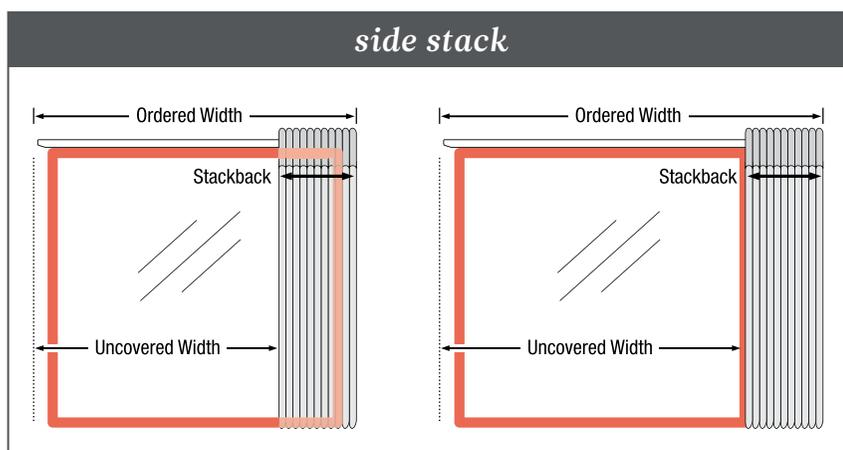
**SIDE OR SPLIT STACK** Shadings can be stacked on the left or right side of a window with the control wand on the stacked side. Or, open shadings from the center with the wand on either side.
