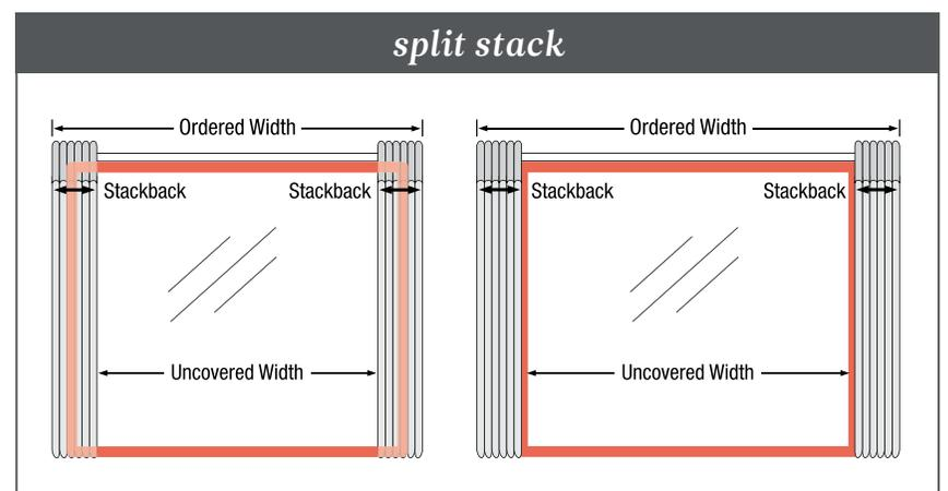
**Stackback** is the width of the fabric panel when the shading is fully drawn. For outside mount, be sure to add this width if you want the shading to stack **completely off** the window or door opening.
