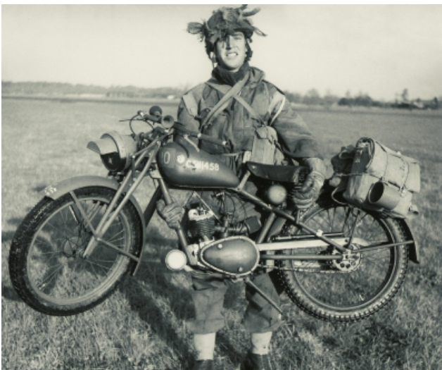
Royal Enfield RE/WD Flying Flea 125 Parachute Motorcycle. It was manufactured at Royal Enfield's underground facility in Westwood, UK, during World War II.
