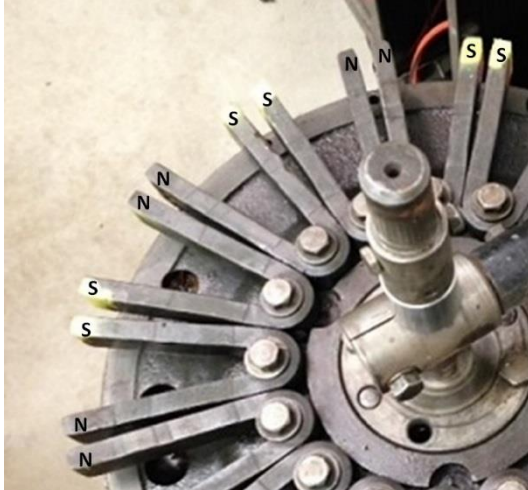
Figure 2. Magnet alignment on the flywheel
