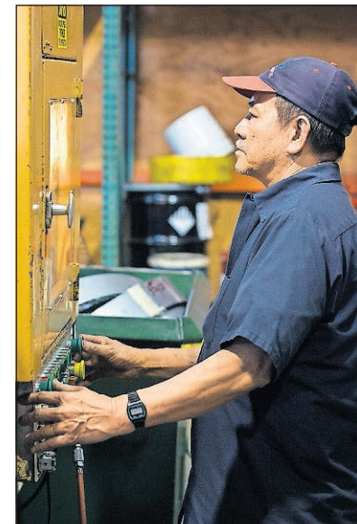
Nguyen Minh watches closely as a machine stamps parts. Swiss Tech Precision USA uses a specialty type of metal stamping called fineblanking that allows it to make massive amounts of intricate parts that can have complex shapes and holes.
