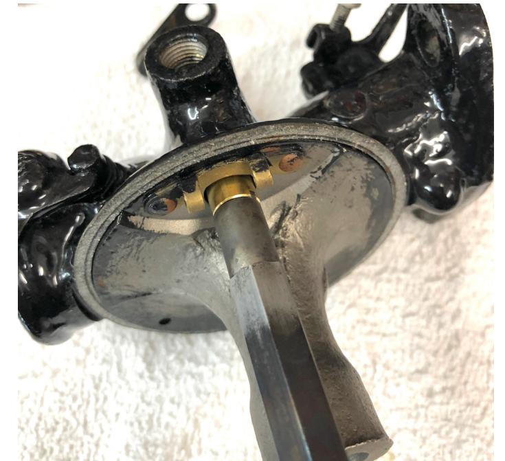
5) Placing the new seat with the insertion tool
