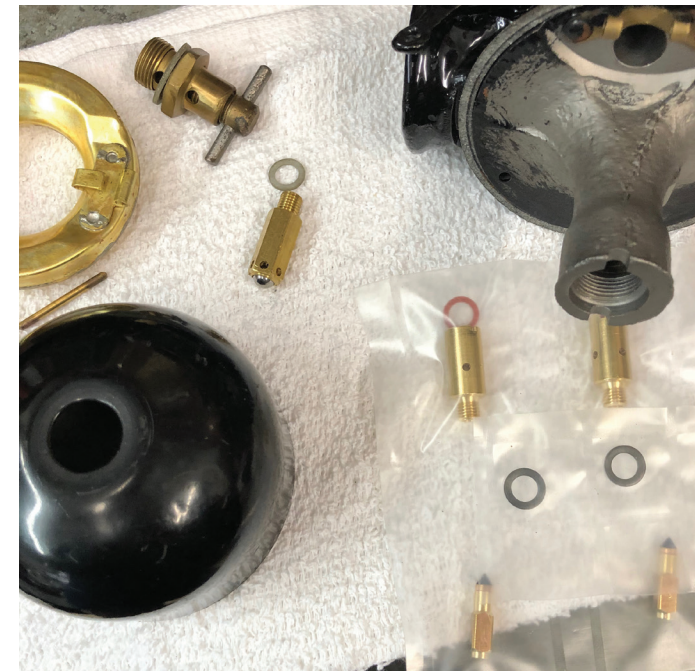
4) The hex-shape Grose seat (upper left) removed, along with its stiff red fiber gasket. New package of Full Flow pieces ready to fit to the Holley NH carburetor.
