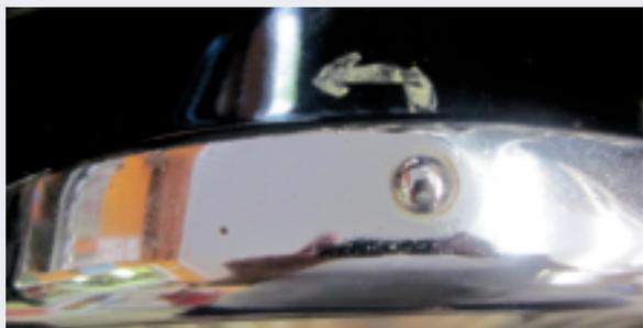
To remove the reflector, pry it out of the bucket, after removing the bulb, by carefully rotating the reflector until the 'cut-out' section is aligned with the grooves in the headlamp bucket edge.
