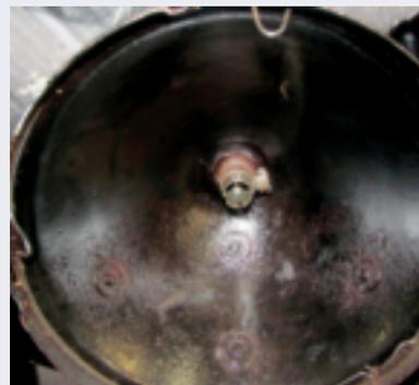
The glass lens should be firm in the rim. If loose, it can rattle. Careful and gentle pressing of the tabs over the glass will secure the lens.
