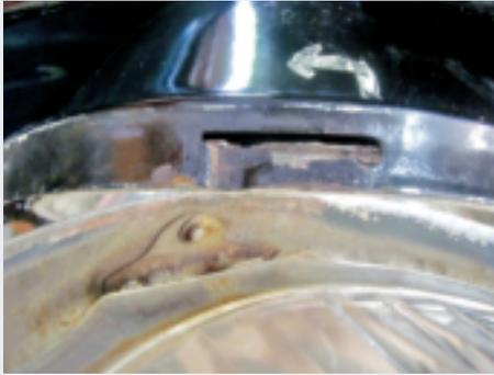
Again, rotate the reflector in the headlamp bucket until the 'cut-out' opening clears the groove, as a solid edge of the reflector should be behind the groove. Replace the bulb.
