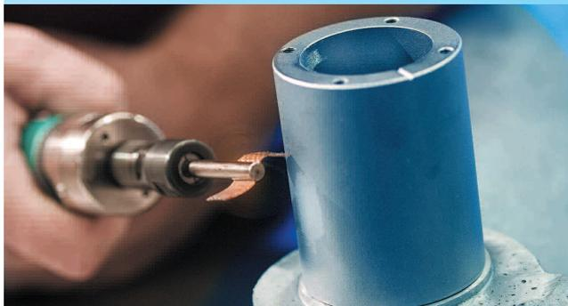
*Flapper peening is ideal for repairing small and hard-to-reach areas. Flapper peening can be done in the field, making the time-consuming and expensive disassembly and transportation of components unnecessary.*
