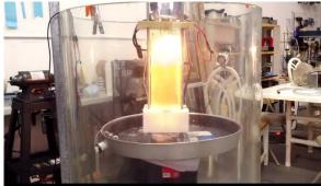
In Run 62 the Plasma vessel will be run by the MM1 Power Generator / Motor producing a low level plasma. A 250 Volt DC potential applied from a lead acid battery array is used.
