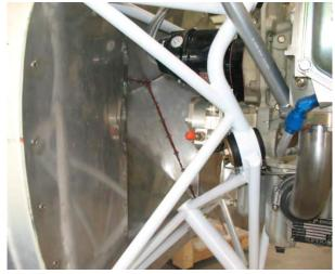
These photos show a close up of a firewall recess area that was required to make space for 0-320 engine accessories.
