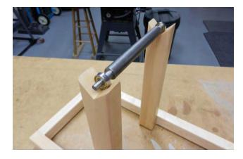
Thanks Gary. Your homemade wheel balancer looks very similar to one that I use that was originally designed to balance go kart racing wheels. Buz
