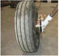
Old nose gear on left; new design in middle with changed socket angle. Right photo is new lower main gear weldment for heavy duty axles and brakes, this is a bolt on type axle, all gear "toe" can be taken care of with shims from Matco.
