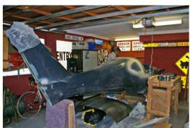
I've fitted a Sensenich 64" ground adjustable prop with a Cummins spun alloy spinner. I also have Skyview 10" display with GPS, MicroAir radio and transponder and an Eflaps push
