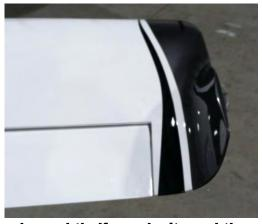
The short "winglet" tips can replace the standard round tip if you don't need the added wing area to meet the "light sport" stall speed.
