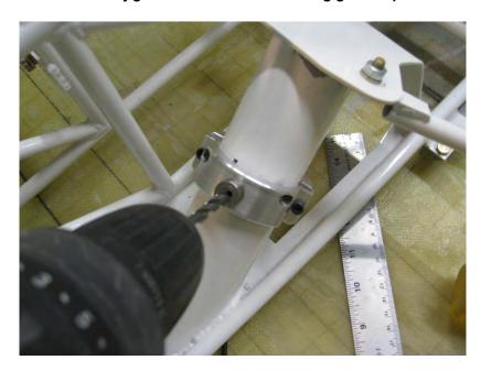
I forgot the "tell" part of "show and tell" on the new and improved choke and throttle bracket. The drill instructions for the throttle lever bracket locate the throttle cable hole too high, not in line with the lever. So, I made a new one from .063" 4130 steel with the top hole 3/8" higher, which lines up more better, less worse.
