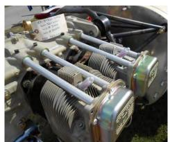
Mark shows off the new 160 HP O-320 Lycoming. This thing is going to be fast. They may need a new airspeed indicator that is calibrated in mach numbers.
