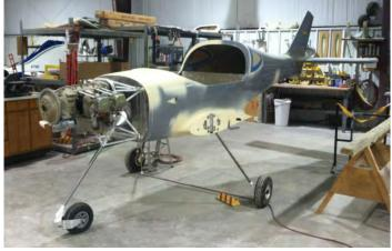
These photos shows the O-320 Lycoming hung on the fuselage. Photo on the right shows the new longer gear legs and the new lower nose socket. The longer gear legs were needed because the 160 HP engine must swing a much larger diameter prop for efficiency (and speed!). That's what its all about – speed.
