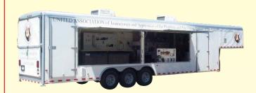
Two entry doors, back loading door, and two side mounted awning doors
