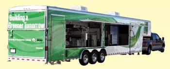
Two entry doors, back loading door, and two side mounted awning doors, and solar mounted roof panels
