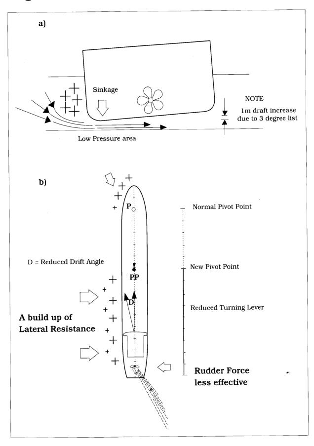
Fig. 13 Turning in Shallow Water
