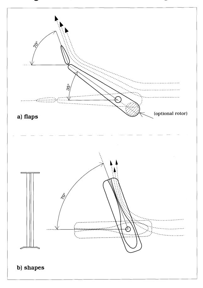
both faces and this creates a positive pressure on one side, but equally important, a negative pressure on the opposite side and this gives the rudder, rather like an aircraft's wing, its lift (see figure 52a).
