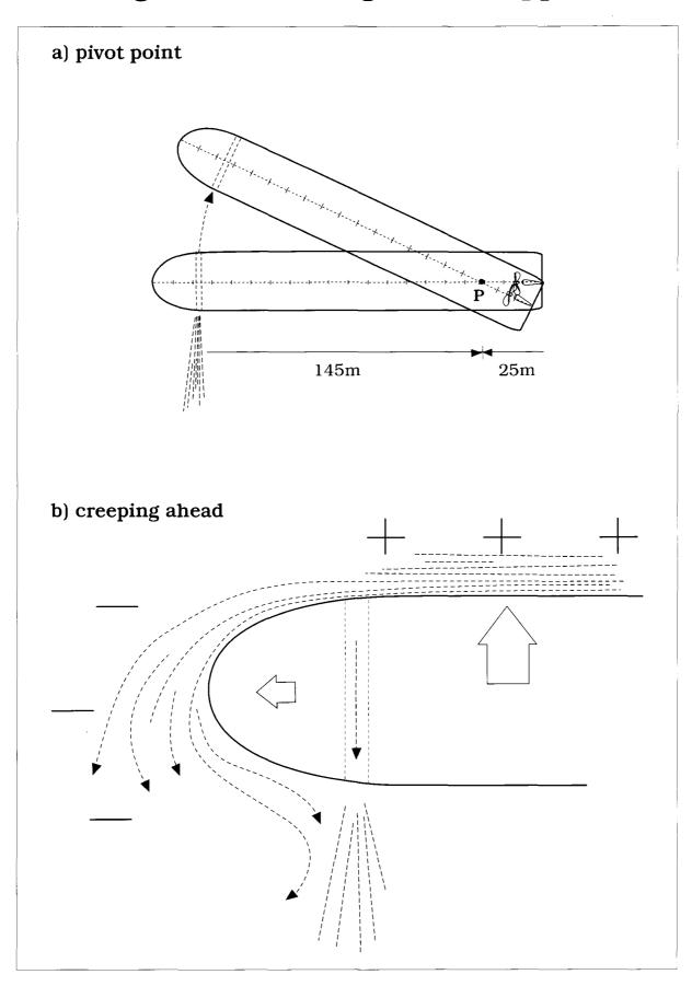
Fig. 44 Thrusting with Headway
