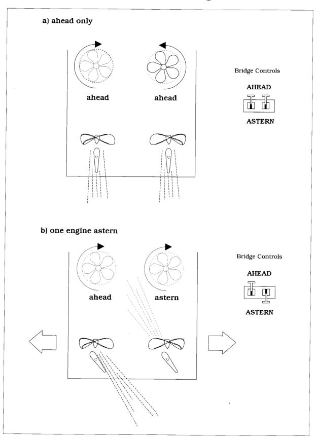
Inward Turning Fixed Pitch Propellers Fig. 57(a) and (b)
