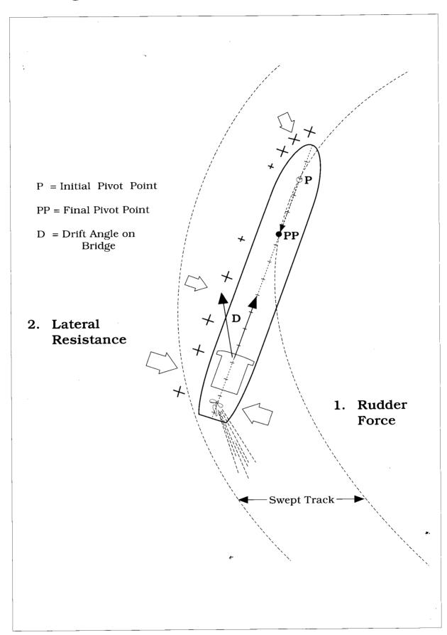
lateral resistance are always achieving the same balance thereby assuring that each turning circle is approximately the same, in terms of advance and transfer. The only thing that is saved by entering a turn at higher speeds is time. It is the 'rate of turn' which varies. Whilst this can be critical in cases when time is of paramount importance, such as conducting a large turn across a strong tide or taking the ship through a 'WiHiamson Turn', it does not improve turning ability.
