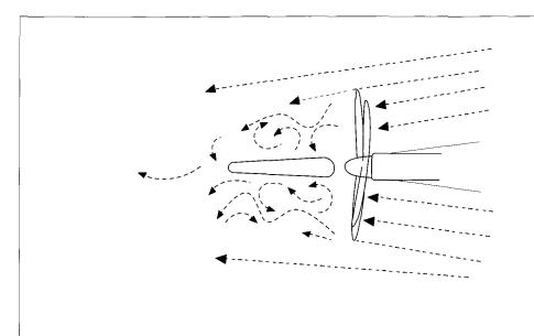
a) impeding the rudder with fine pitch settings
