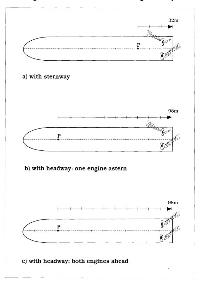
Turning ability at speed Fig. 58(c)
