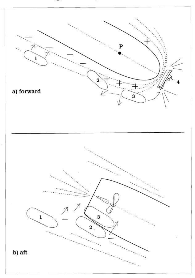
by the flow of water into the propeller aperture whilst the engine is turning ahead and, it should be noted, at any time whilst controllable pitch propellers are engaged.
