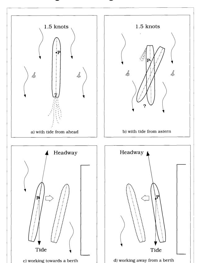
By working the ship across a tidal stream in this manner, the tide is really being used as a sort of 'poor man's tug' and in tidal work, more than anywhere else, the ship handler needs to develop a keen, sensitive 'feel' for the movement of the ship, virtually drifting it into the desired position.
