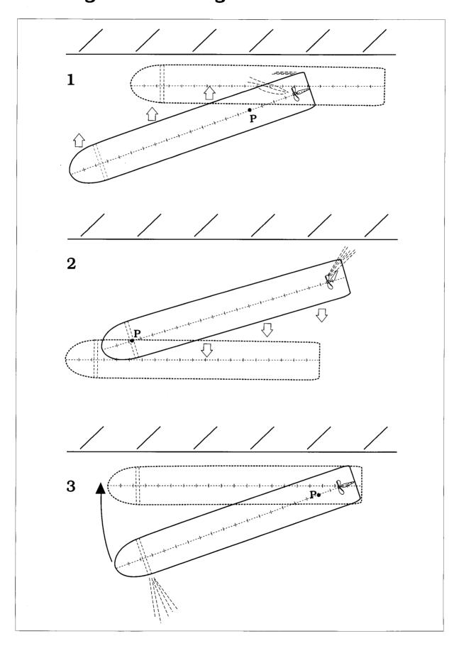
(It is not uncommon during this manoeuvre for large ships to engage one tug - which is secured aft - where it can assist very effectively with the steering and positioning of the stern, whilst the bow is controlled solely with the thrus ter.)
