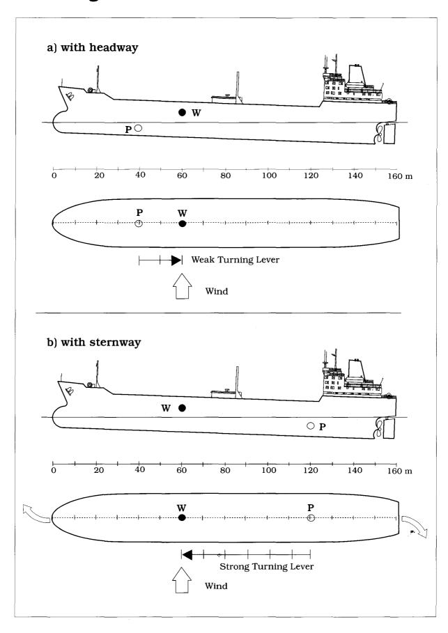
well ahead as such a ship can prove very difficult to hold in position. However, as long as we have some prior knowledge as to how the ship will react, under the influence of the wind, it can be turned to advantage and readily employed to aid rather than hinder ship handling. Not for nothing is it often referred to as a "poor man's tug!"
