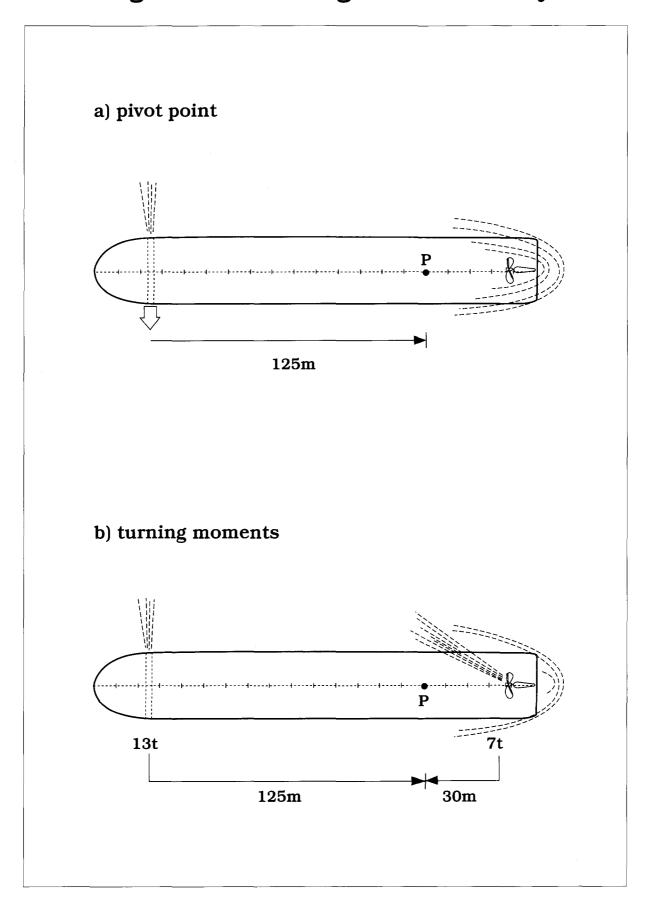
point has moved aft to a position approximately a 1/4 of the ships length from the stern (see figure 47a) and the bow thruster can now work on a respectable turning lever, in this case 125m.
