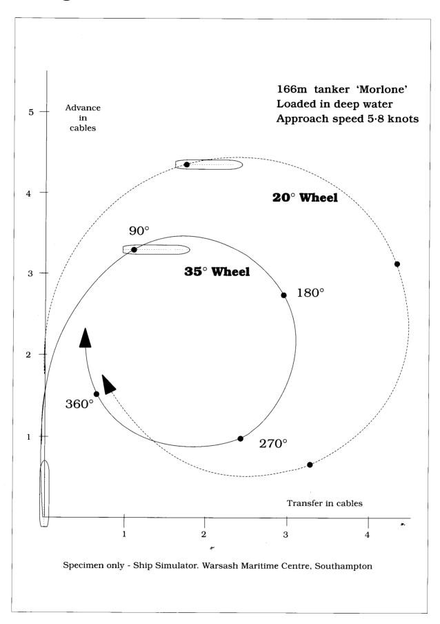
Fig. 9 Full Ahead Turns to Starboard
