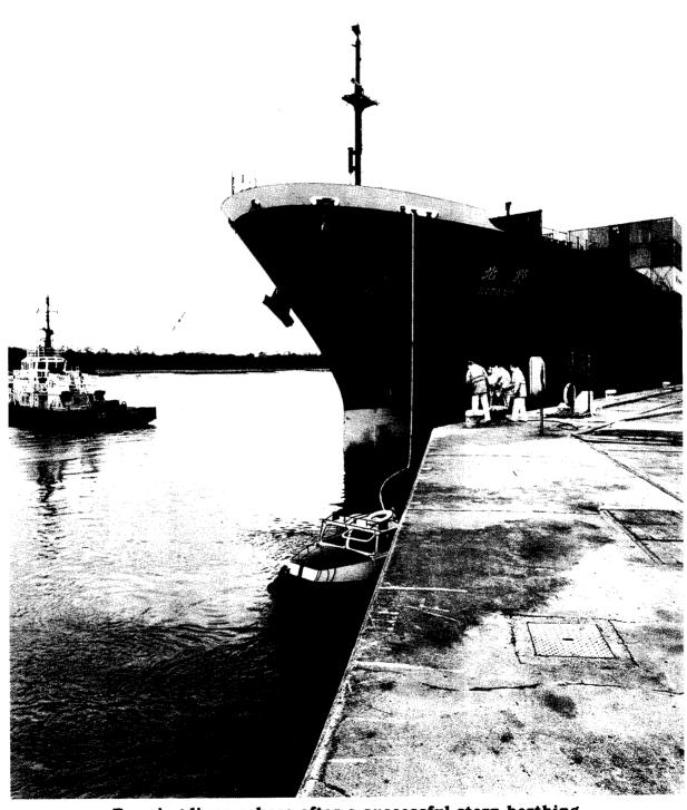
Running lines ashore after a successful stern berthing using tugs and thruster combined
