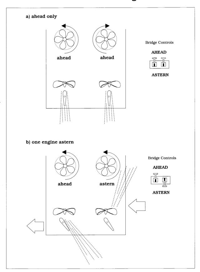
Fig. 57 Twin Fixed Pitch Propellers — **Inward Turning**
