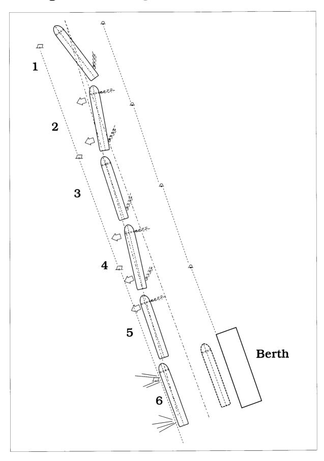
Fig. 49 Working Astern to a Berth
