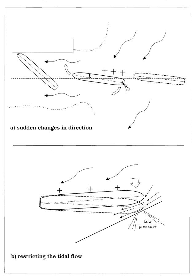
it is still working strongly on the starboard quarter. With the combination of slow speed and the pivot point forward, the tide aft is working on a good turning lever. This creates a strong turning moment and the bow, which was already canted that way, will swing rapidly to starboard. It is therefore important to anticipate this and check it immediately, with a substantial kick ahead.
