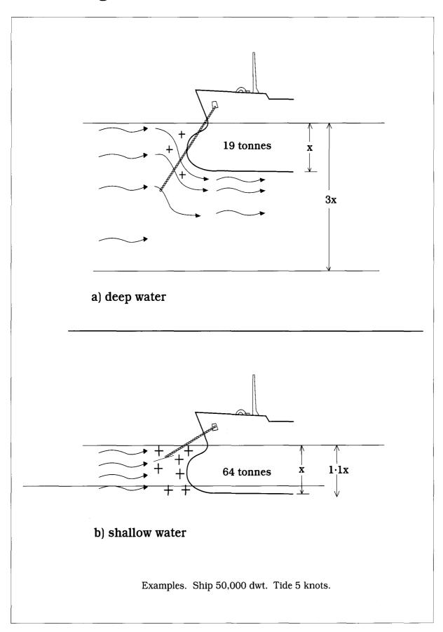
This is an extremely important point, because the force of a strong tide over the period of dead low water could just exceed the holding power of the anchor and the ship will drag, particularly if the ship is laying to a strong wind as well!
