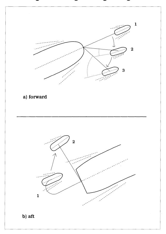
as shown in position 1, figure 63b. However it can, if it is safe to do so, move out to position 2 or thereabouts and 'lay' on the tow line with its own weight, but unfortunately it must keep the tow line aft of the towing hook position. Under the circumstances this design feature seriously limits the tug's arc of operation.
