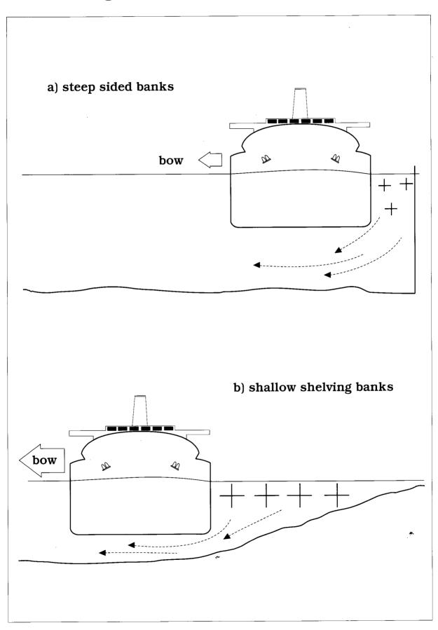
longitudinal resistance and pushes the pivot point back from P to PP and the steering lever is reduced (see figure 26b). The ship will now 'squat by the bow' which in turn makes the problem even worse. Several cases have been reported of large ships running in shallow water and experiencing bow sinkage of up to 2 metres!
