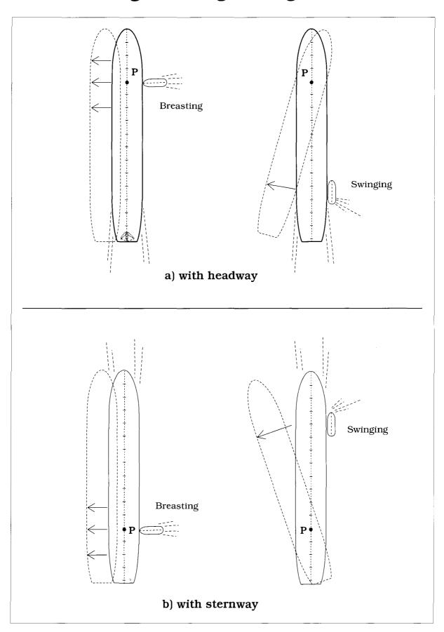
If the tug is used aft, as depicted with the ship on the right in figure 71a, its role is very much altered. Wherever it is placed it is likely to be some distance from the ship's pivot point, working on a substantial turning lever and as such will always be best placed to help increase or decrease the ship's rate of turn, whilst making headway.
