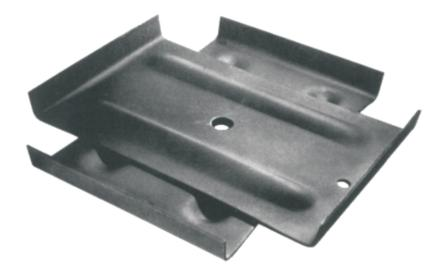
Cross-Plate anchors are formed from structural steel and are ribbed for extra strength and reinforcement. Plate edges are flanged to resist creeping. Plates are welded at right angles for maximum holding ability. Nut retainer is provided to aid installation.
