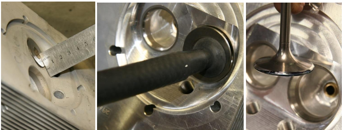
Figure 95 – Recessed Valve Seat, Valve Being Cut
