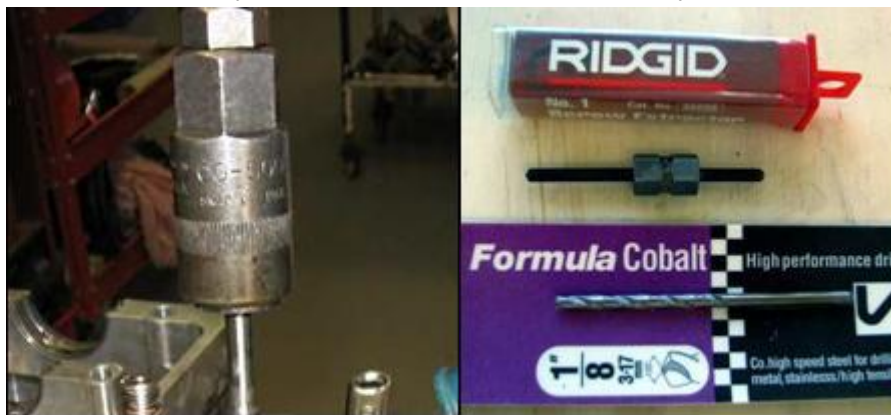
Figure 63 – Stud & Broken Cap Screw Removal
