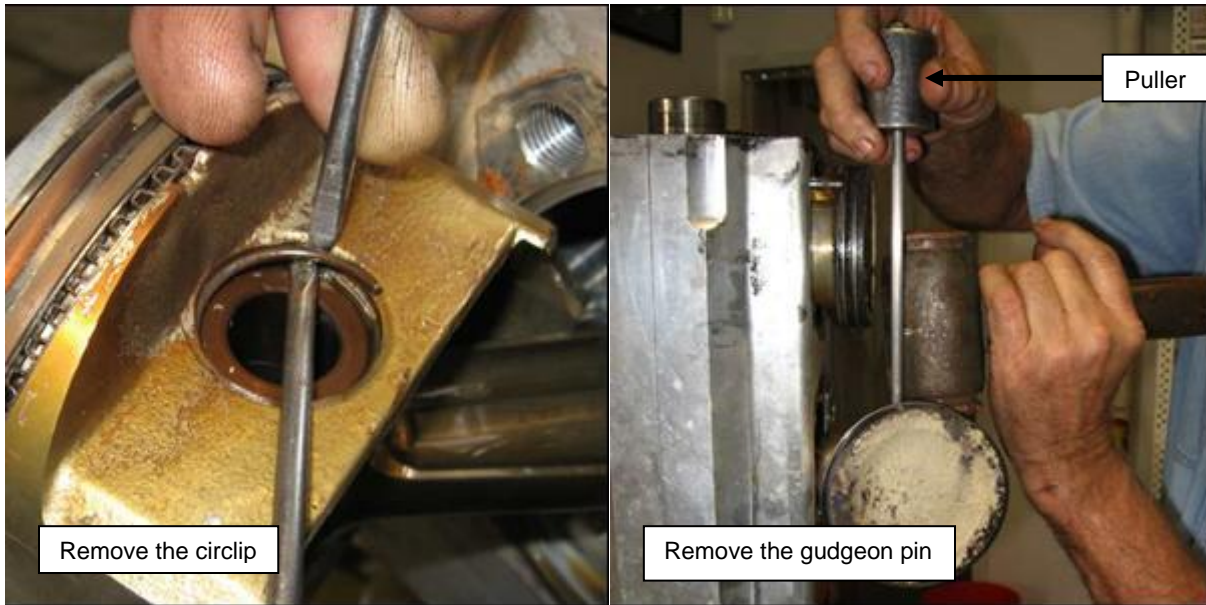
Figure 55 – Remove Pistons
