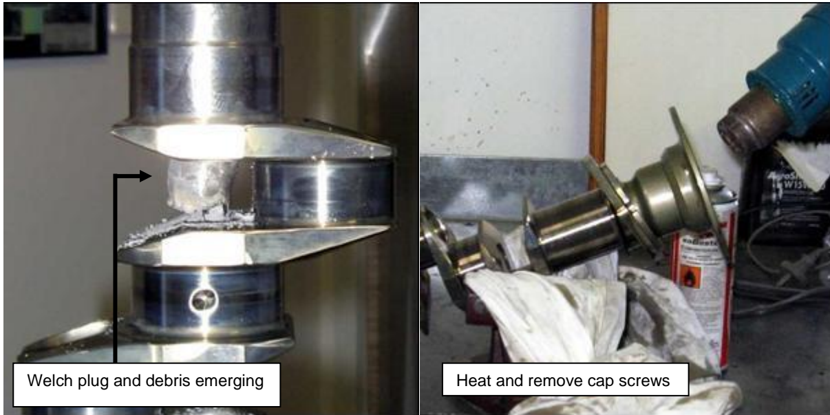
Figure 62 – Welch Plug & Propeller Flange Removal From Crankshaft
