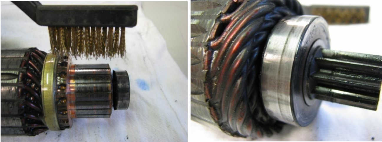
Figure 110 – Starter Motor Overhauling
