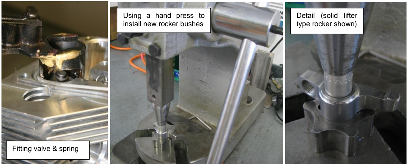
Figure 148 – Fitting Valves to Head, Fitting Bushes to Rockers
