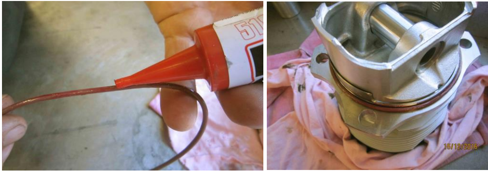
Figure 162 – Applying Sealant and O-Ring to Cylinder Base
