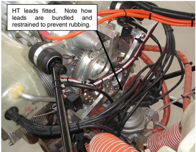
Figure 203 – HT Leads Fitted To Engine
