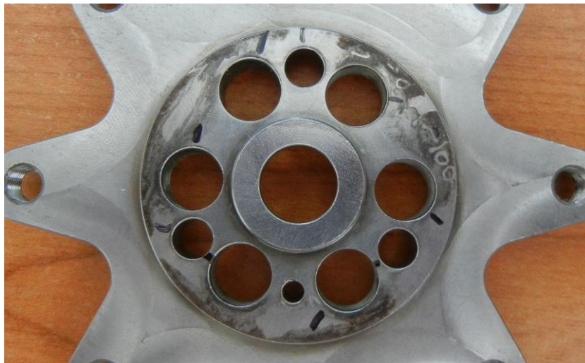
Figure 106 – Damaged Flywheel “Starfish”
