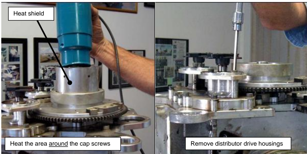
Figure 48 – Removing Flywheel Cap Screws & Distributor Drive Housings
