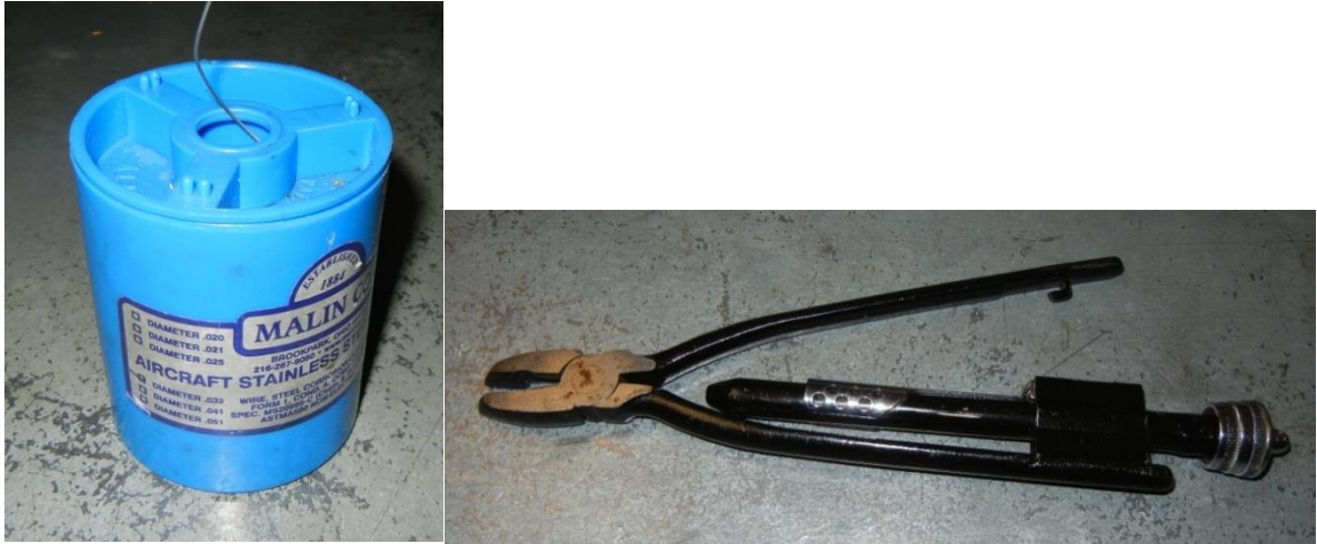
Figure 9 – Safety Wire / Wire Pliers
