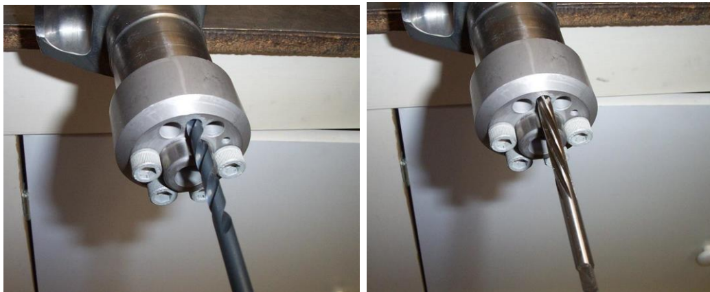
Figure 220 – Drilling & Reaming Crankshaft – ILLUSTRATION ONLY.
