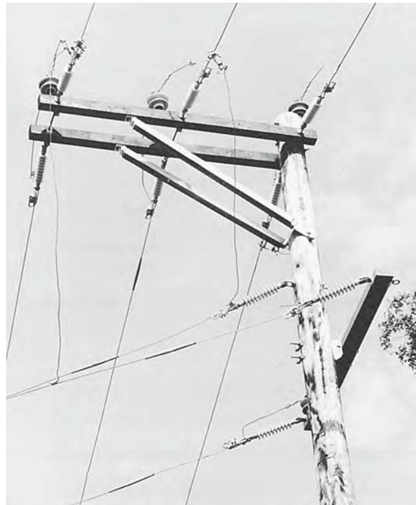
Come complete with lineman's step. For applications where step is NOT required, add suffix-L/S to catalog number. Alley Arm braces are supplied in the traditional style (AAB series) or Reversible style (RAAB series). Alley Arm Braces are made of high strength 2 11/16" x 2 11/16" 'apitong' wood and "boltless" aluminum end fittings. End fittings are normally supplied containing a 11/16" dia. mounting hole.
