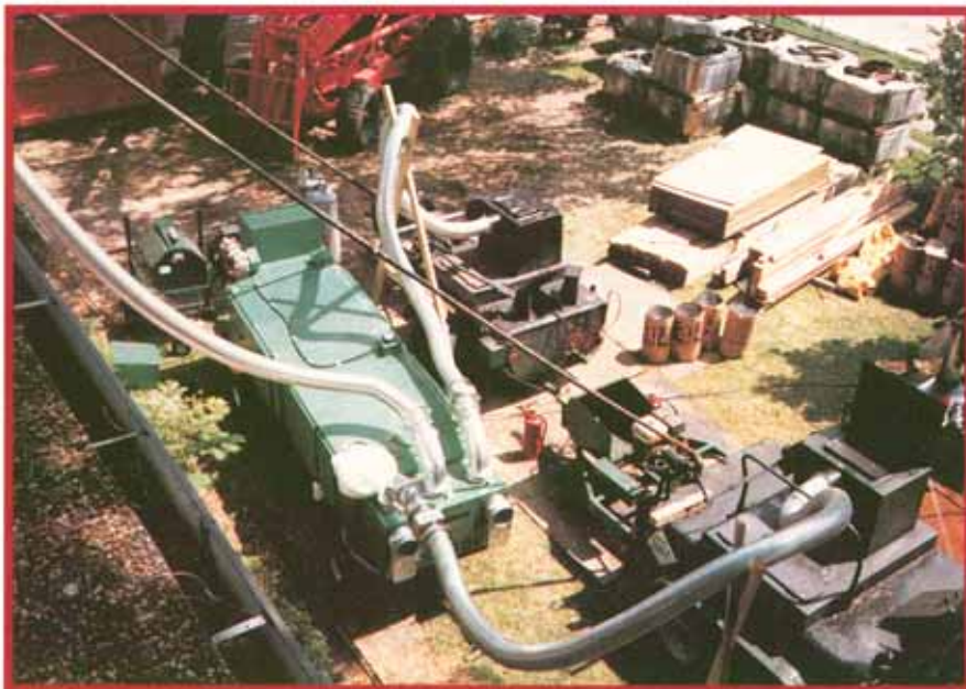
The FRS-6000 draws the fumes through the flexible hose and into the filter chamber where 99 percent of the particulate matter is removed.
