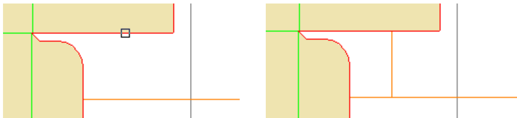
Fig 41 - Intersect Strip Knife Option disabled (left) and enabled (right) for an external waste area
