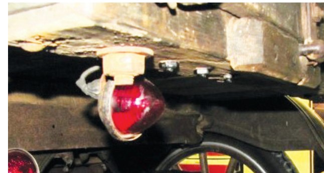
Clearance lamps mounted under my wood Pickup bed, one on each side. They are wired to a switch connected to the brake pedal. . . . .
