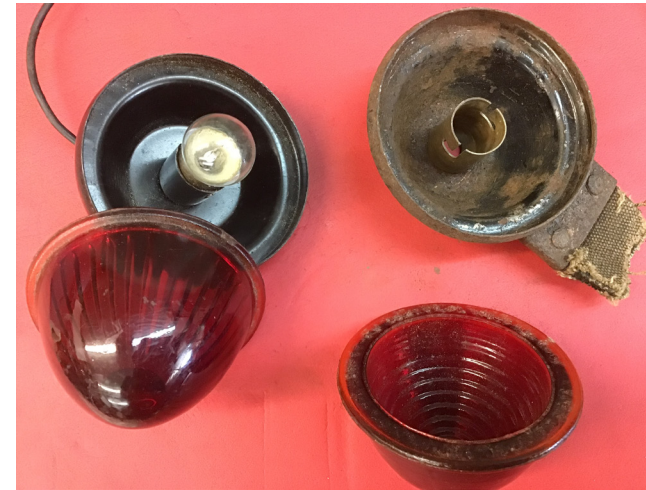
Newer and vintage clearance lamps suitable for tail lamp or stop lamp use
