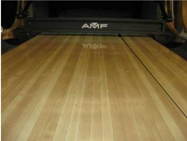
2. Adjust first guard height over the lane with threaded link (about 1.25" off lane),
