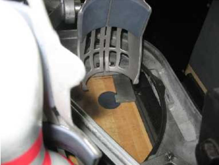
Once you have achieved 5/16"-parallel, then check the table centering with table flags. Center the table over the Pindeck Spots, both front-to-back and right-to-left – within 1/16" in each direction.
