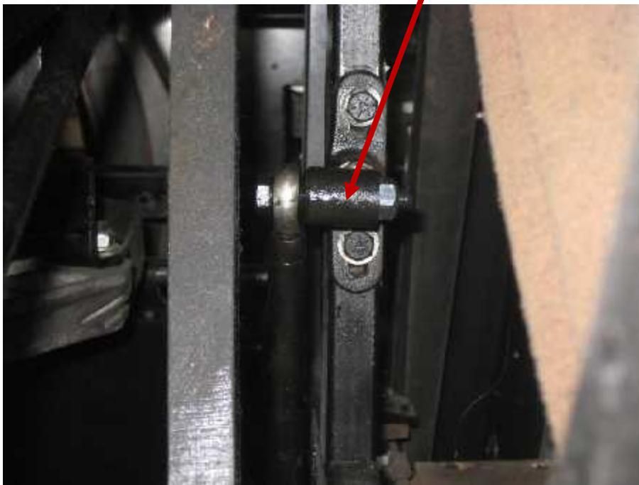
Turn the Threaded Link SHORTER to LOWER the guard position, and LONGER to raise the guard position. Make sure that the Threaded Link is parallel to the lane after retightening.
