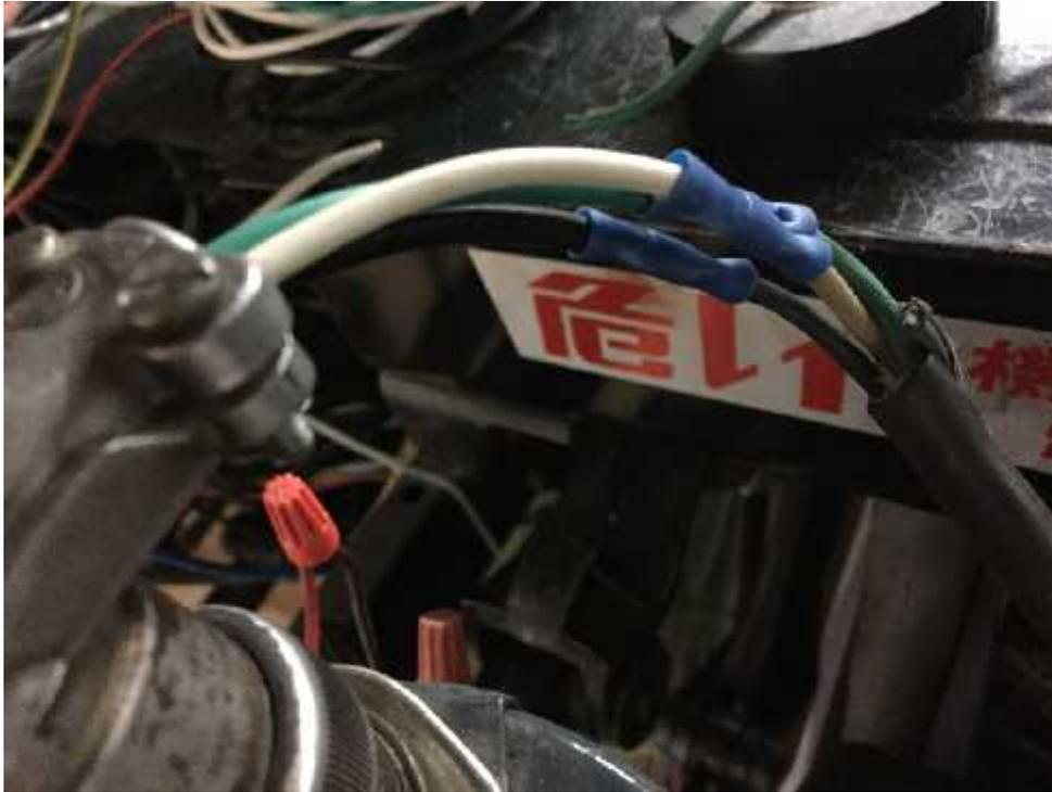
The C1 and C2A plugs are broken, exposing hot wires to shorting-out possibilities.
