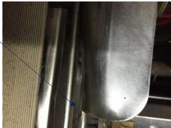
As we were correcting this issue, we noticed that the plow on the 10-side of this lane was SO LOW, that it was wearing-out the carpet and causing the back end motor to quit working. We adjusted the plow to the correct height.
