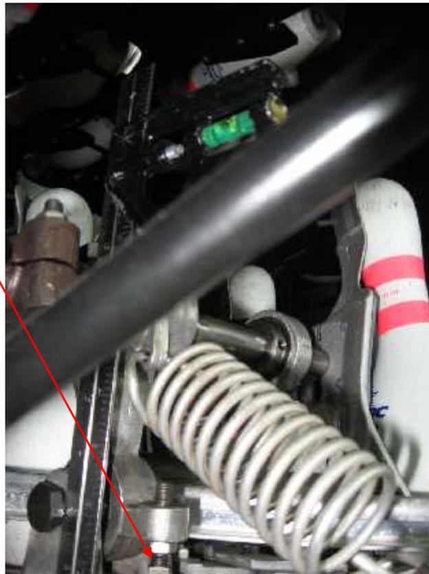
5. Crank table forward/down, until pin bottoms are hovering over pin spots, and adjust cup sizes for even hang. Adjust spot rod for proper "toe," (slight clearance between the square head stop bolt and the stop – so that ANY downward pressure on the table causes this gap to widen):
