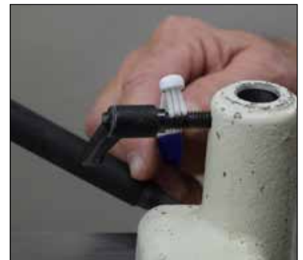
Picture #20 - 1414 Caption - Use a stiff brush to clean the threads of the tool rest clamp.
