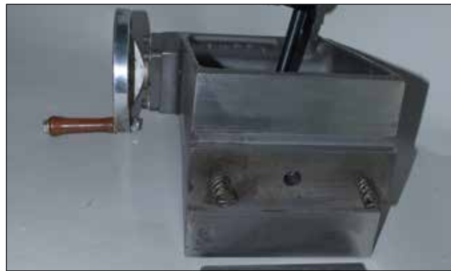
Picture #25 - 1433 Caption - Some lathes will have rectangular locking plates and springs.
