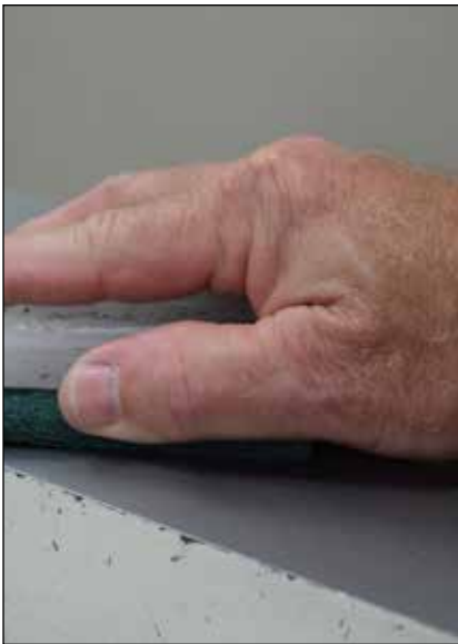
Picture # 10 - 1377 dupe Caption - Load a non-woven abrasive with wax and apply to the top and side surfaces of the ways, but not the bottom.
