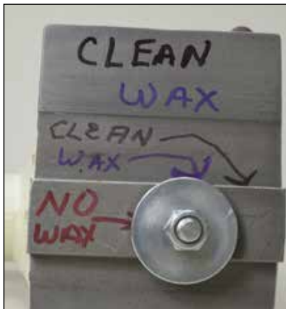
Picture #26 - 1473 Note to editor. Use # 1440 with typing in lieu of my printing. Caption - After cleaning, lubricate the tailstock surfaces that make contact with the ways.
