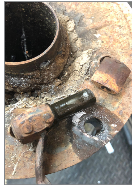
Old camshaft and lever removed
