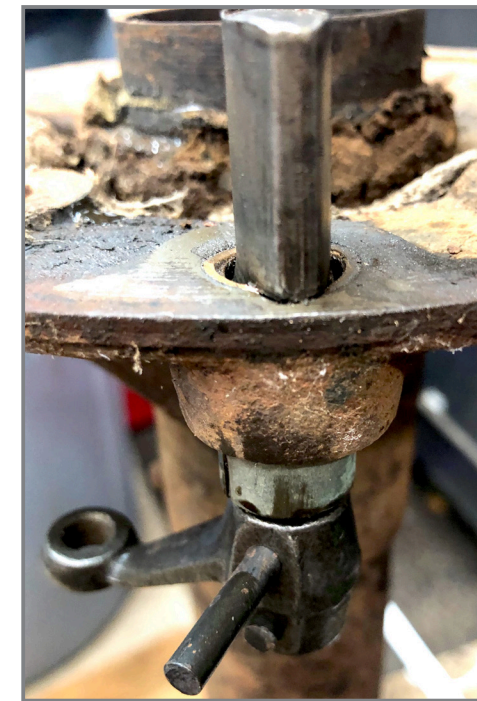
NOS lever and camshaft rivet going in place
