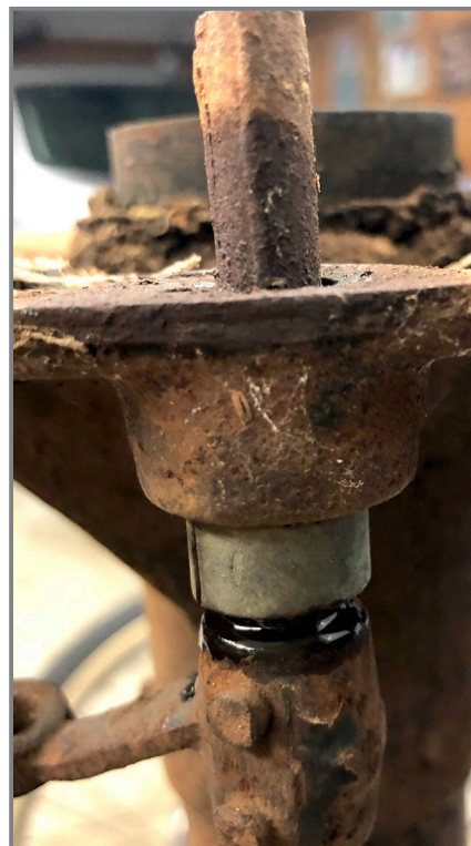
Using penetrating oil to free up the camshaft
