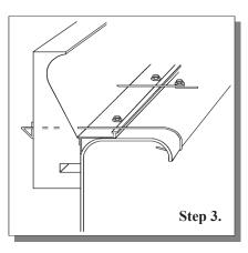
**Step 3.** Push the tie wire through the form even with the top of plumb strip. Wrap the end of the tie wire around the screw, while applying slight pressure.
