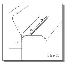
**Step 2.** Peel the paper off the tape. Stick the form to the plumb strip and pool wall, with the lower edge of the form profile even with the top of the plumb strip.
