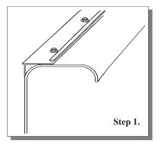
**Step 1.** Place the Plumb Strip so that it makes the transition from pool wall to top lip square and screw it down.
