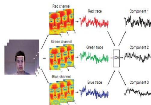
Fig. 3: Feature Extracted in Component based algorithm
