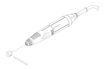
• Insert the 1.5 mm hexagon key wrench through the hole located on top of the chuck tool. Insert the key wrench as far as it will go into the chuck. The key wrench will come in contact with the micro adjustment screw at the very bottom of the chuck. Keep the chuck tool still and turn the wrench counter-clockwise;
