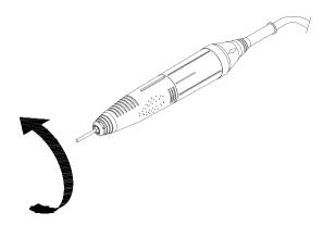
• Insert the chuck tool into the chuck itself. Insert the pin in the side hole of the chuck tool to act as a lever. Please note: The pin used as a lever in this step is the pin that was in the micromotor's chuck assembly when you received and unpacked your iON;
