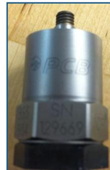
FIGURE 8 - PCB ACCELEROMETER FOR RESPONSE AND REFERENCE
