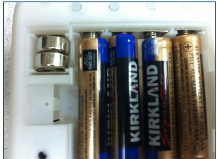
FIGURE 12 - POWDERING ON BATTERIES
