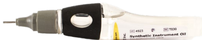
12 ml Synthetic Oil Pen T030 To avoid fretting corrosion Apply a drop of lubricant after cleaning and before sterilization on all joints, threads, and sliding surfaces
